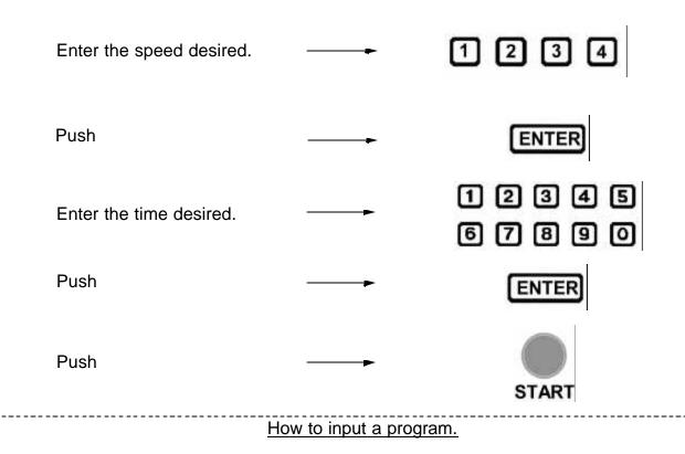
A flashing display indicates that it is expecting the operator to key in a value.
